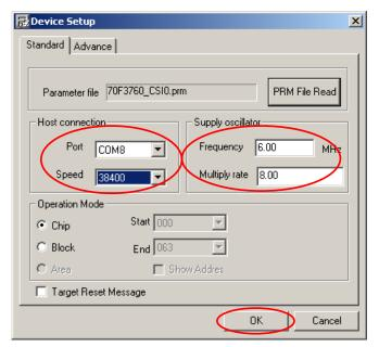
"Port" selects the COM port number where TK-850/JG3H is allocated.
