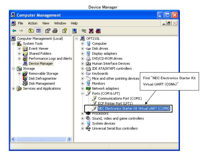
The screen above shows that the COM port number is "COM8". If ID850QB is not in use, you can use this port number for connecting TK-850/JG3H.
