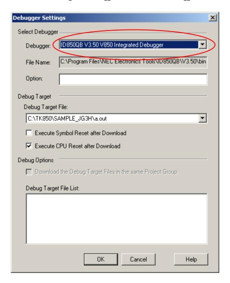
If you cannot select "ID850QB V3.50 V850 Integrated Debugger", select "Project" on menu bar, "Project settings" -> "Tool version settings" -> "Detailsetting" -> then select "ID850QB V3.50".
