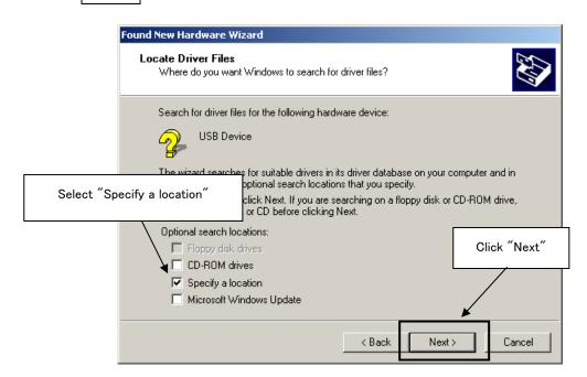
4. Select the driver directory path. The path should be "C:\text{Program Files}\text{NEC Electronics Tools}\text{TK-driver" as default installation.
