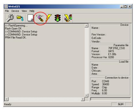
Terase The deletion of the flash memory begins when the button is pushed.
