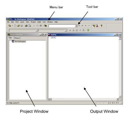
Project window A window in which project names, source files, and include file are displayed using a tree
