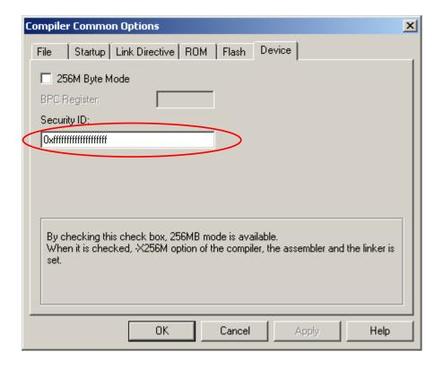
Set the security ID. The security ID is a specific ID code (10 bytes) used for the authentication when the debugger is starting. The security ID is stored at the address 70H-79H in the microcontroller built—in flash memory. The security ID in the flash memory and the ID entered in the configuration dialog are compared when the debugger is starting. When the ID does not match, the debugger cannot be started. Therefore, it is useful to protect the program data in the memory from others.
