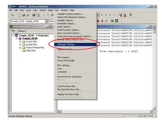
Check if "ID850QB V3.50 V850 Integrated Debugger" is selected on "Debugger".
